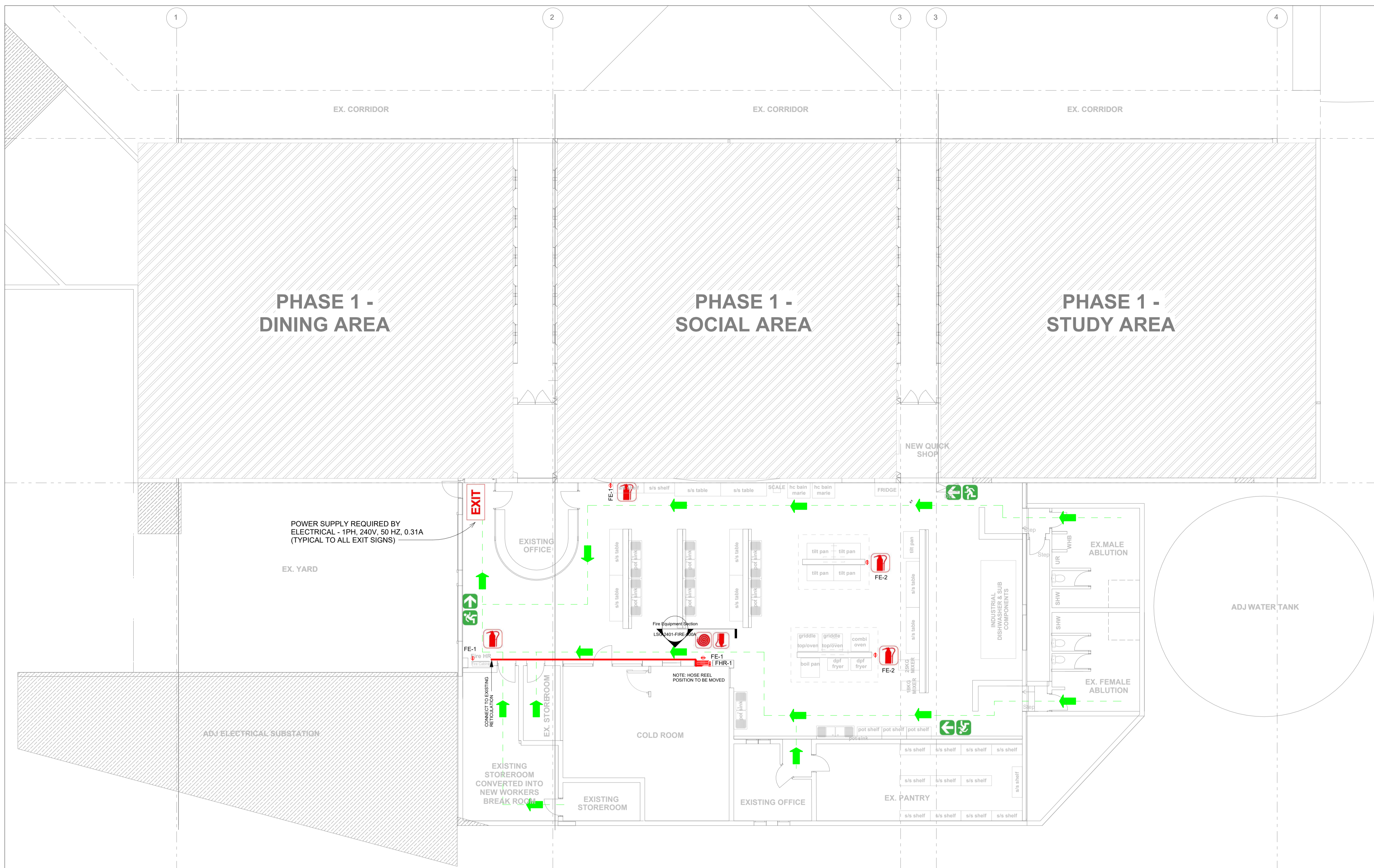
1 Fire Protection Layout - Consolidated Ground Floor 1 : 100
